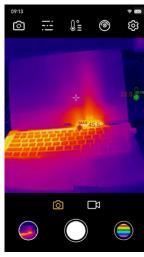
3. To make an accurate measurement, you must properly set the parameters. For example EMS, distance, ambient temperature, and others. See below and refer to the help file in the APP.
